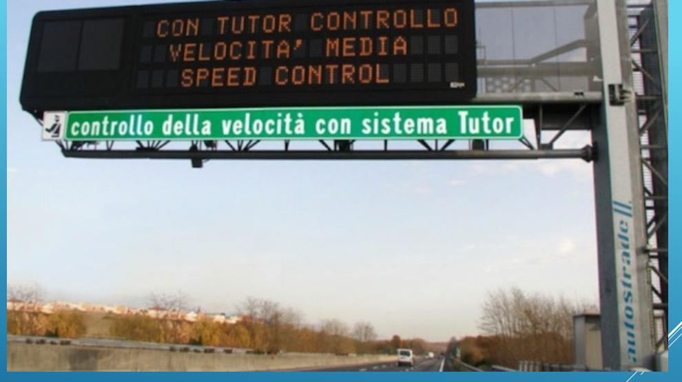
The Speed Control with Tutor System can measure the "instant" speed as the vehicle passes or they can average the speed of the vehicle in a stretch of road between two detection stations.
